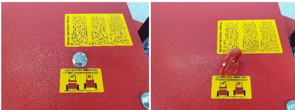
This model has 2 counterweight layers of approx. 600 kg each. You can lift these from the machine with 4 lifting eyes supplied. Screw these lifting eyes into the holes provided. (see photo). This way you can only lift the weight package and **not** the entire machine.
