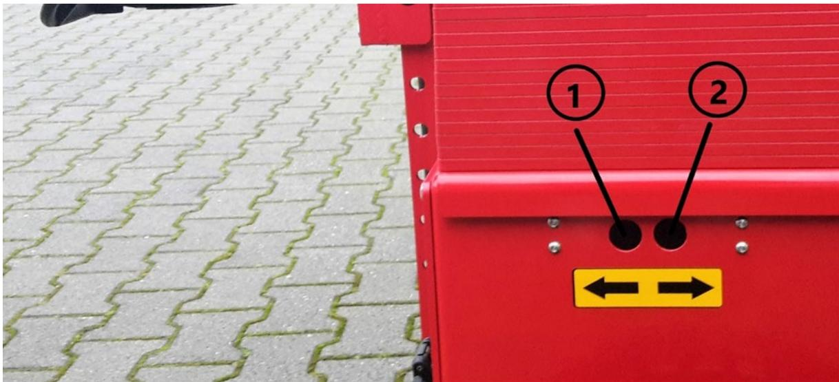
At the front left there are 2 buttons for moving slowly forwards (Fig 3, 1) and backwards (Fig 3, 2). Press the button 1 time to unlock, pressing the button the second time you can drive a couple of inches forward or backward. The maximum speed can be set using the potentiometers (Fig 2, 7 and 8) on the tiller head. The maximum distance you can travel in this way is approx. 1 metre.
